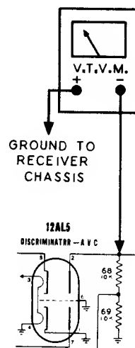
FIG. 3 VTVM Connections for IF Alignment
